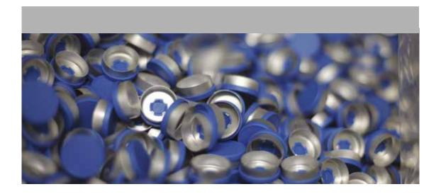
This range of closures is suitable for sealing single-dose and small bottles of medicine which are used with needle and are the most popular on the market. The closures are produced under controlled conditions. During the procedure, the closures are inspected using in-line inspection systems in order to guarantee an optimal product quality.
